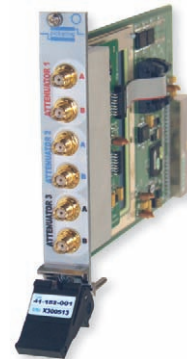
41-182 3-Channel Attenuator 32dB, 0.25dB Steps
